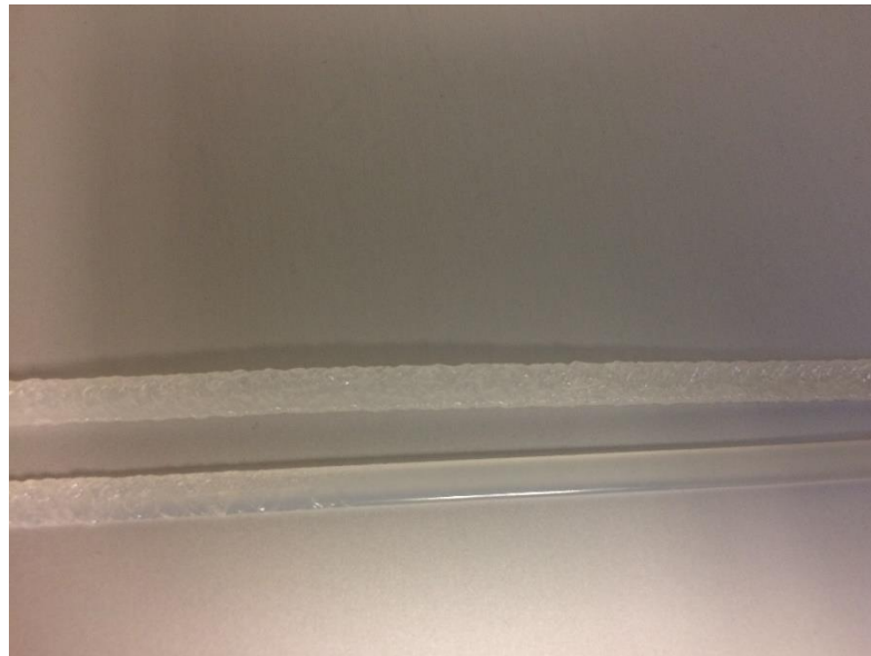
Figure 2-2 Wet nylon (top) vs dry nylon (bottom)
