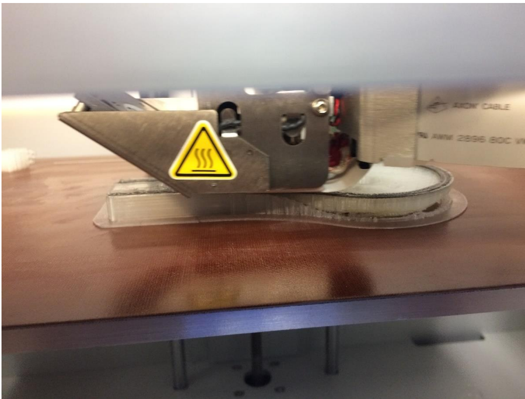
Figure 3-1 Printing a carbon fiber layer
